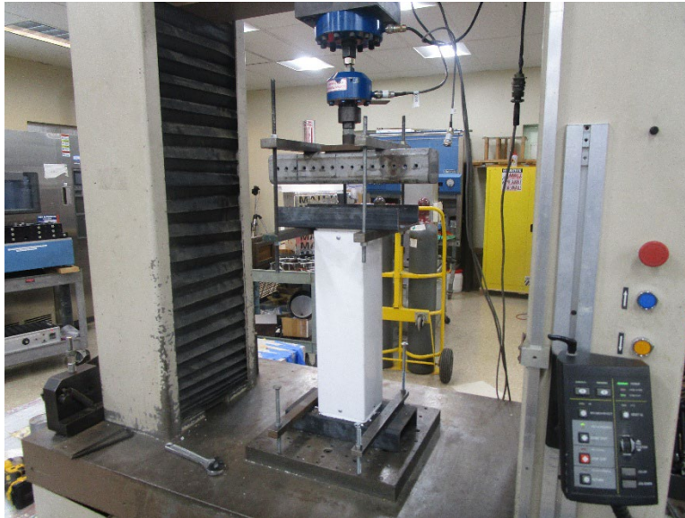
Photo No. 3 Typical Uplift Test Setup
