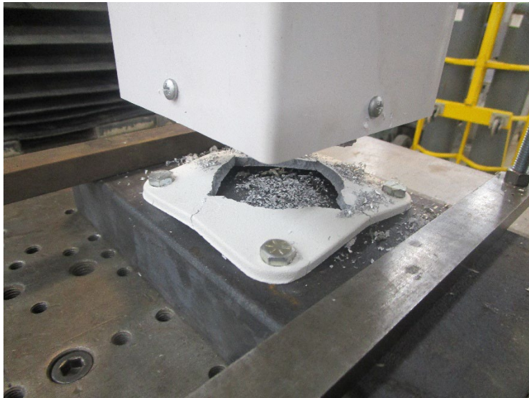
Photo No. 4 Typical Uplift Test Failure
