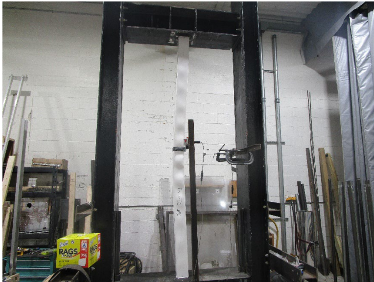
Photo No. 2 Axial Load Compression Test - Buckling Failure
