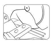
Leave aluminum in while cutting. Make first cut, then slide aluminum ¼" in from first cut before making second cut.
