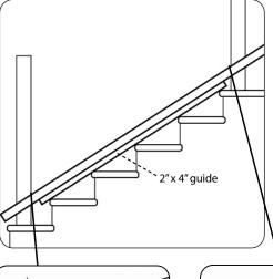
Place a 2" x 4" on the steps – this will be your guide for the bottom rail length and angle of cut.
