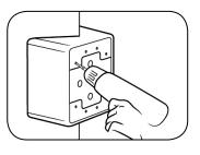
Note: 45° brackets mount on the corners of your post and 22.5° brackets mount on the face of the post.
