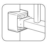
Place external molded brackets onto bottom rail and assemble your rail section per instructions included with those sections - using the 2 1/2" mounting screws included with the angled adaptor block kit. The external molded brackets are designed to allow mounting after the section is located in the molded brackets.
