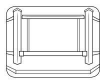
To ensure accurate placement of top angle adaptor block place a baluster from the rail kit into each end of the bottom rail and place top rail in position. Place external bracket on ends of rail. Mark position for angled adaptor block. **IMPORTANT:** Double check that the height of rail is at least 36" or 42" to top of rail. Adjust as necessary.
