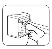
Assemble per instructions included with those sections – using the 2 1/2" mounting screws included with the angled brackets kit attach external molded bracket and rail section to the angle bracket which is mounted to post. Put covers over screws.
