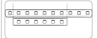
Using the bottom rail as your guide, mark the cuts of the top rail with pencil
