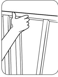
1. Lay the bottom rail (F) onto a clean surface, such as the carton from your railings. With the baluster holes facing up, install balusters (J) into the bottom rail.
