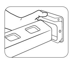
Place rail brackets on ends of bottom rail.
