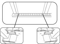
Lay bottom rail in front of post and mark rail for proper cutting on both ends.
