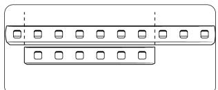
Using the bottom rail as your guide, mark the cuts of the top rail with pencil
