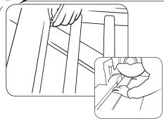
Mark brace to fit snug when placed diagonally between gate posts.
