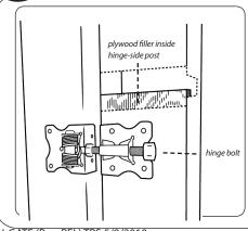
ezTIP: Before installing hinges, determine which way you want gate to swing. Hinges and latch striker will be mounted on the same side of gate posts.
